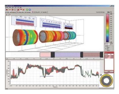
Graphical representation of the monitored objects caused the most difficulties for implementation. We decided to show 3D image of the kiln with infrared picture on its surface. User can monitor calculated thickness of bricks and coating also by the means of sections. We use OpenGL for 3D modeling.
